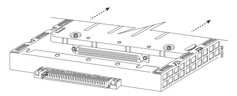
Step 8 If you removed a port adapter, place it in an antistatic container for safe storage or shipment back to the factory. If you removed a blank port adapter, no special handling is required; however, store the blank port adapter for potential future use.
